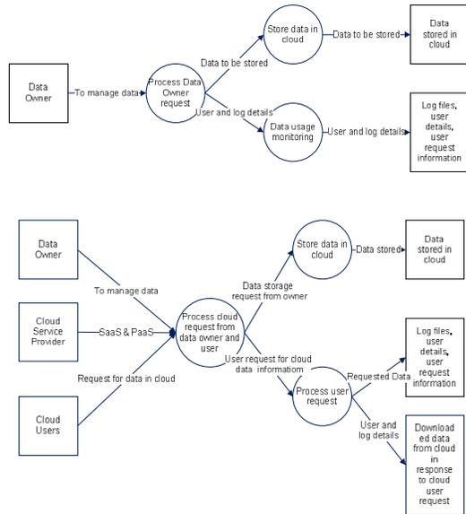
Fig 4.2: Level 1 diagram for data owner, cloud service provide and users process
