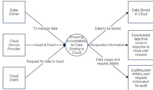
Fig 4.1: Context level diagram for ensuring accountability for data sharing in the cloud
