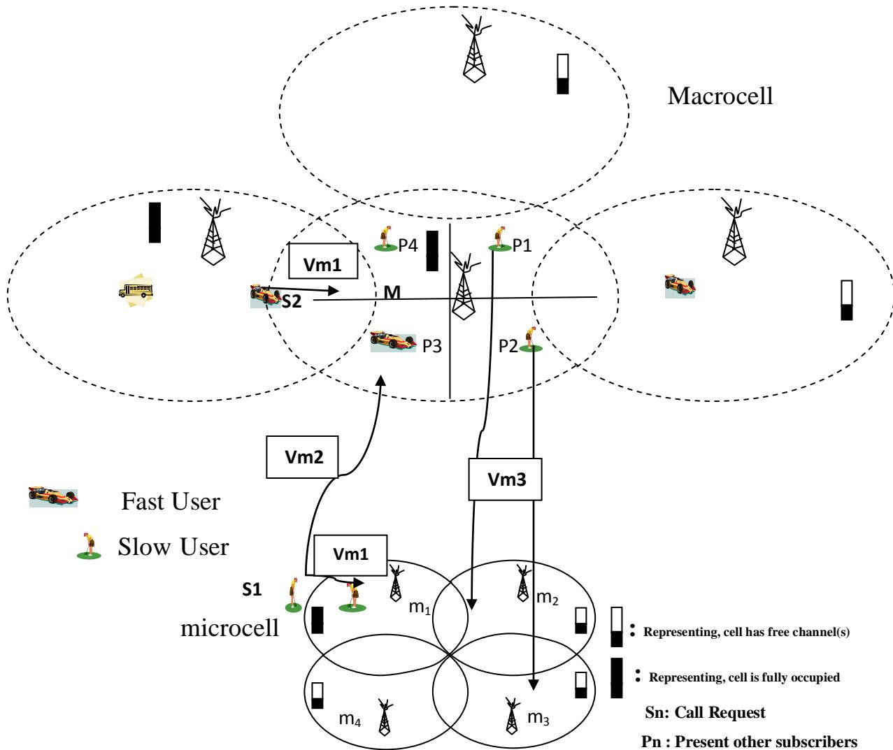
Figure 3: Channel sharing in the vertical direction for slow users
