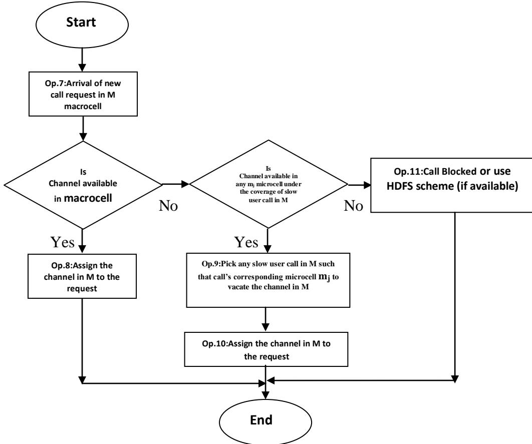
Figure 2: Flowchart ‘B’ showing Operations occurred on Call request arrived to macrocell
