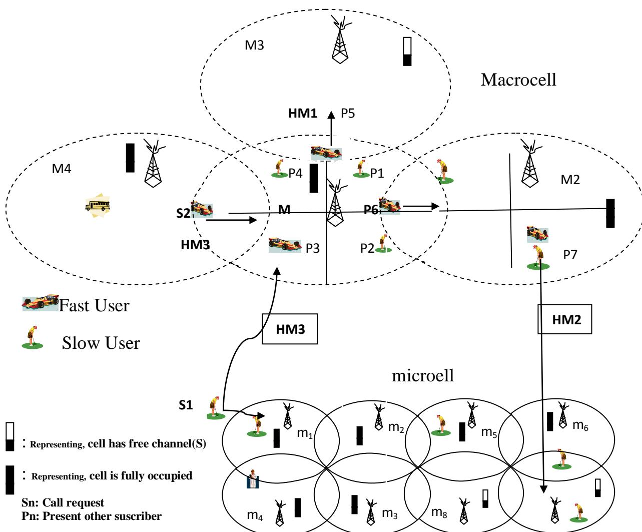
Figure 5: Channel sharing in the horizontal direction for slow subscribers and fast subscribers
