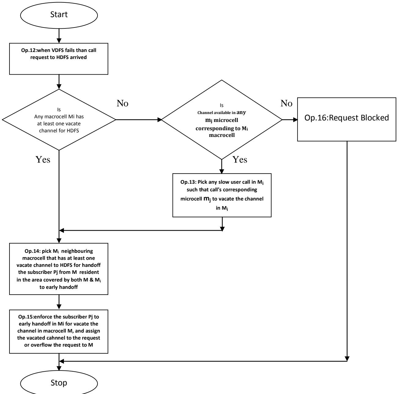
Figure 4: Flowchart 'C' showing Operations occurred on Call request to HDFS
