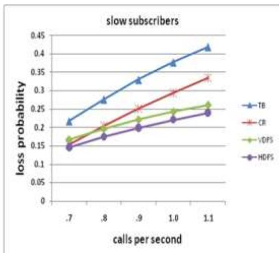
Figure 10: Comparison of numerical analysis on call loss probability with (.7 to 1.1) call arrival rate for slow subscribers
