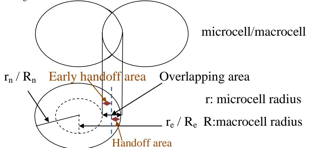
Figure 6: Radii of the circles for the subscribers to take normal handoff and an early handoff
