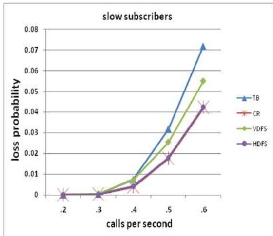
Figure 8: Comparison of numerical analysis on call loss probability with (.2 to.6) call arrival rate for slow subscribers
