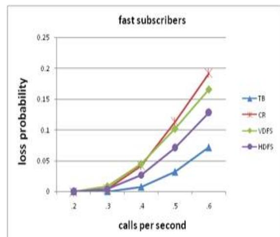
Figure 7: Comparison of numerical analysis on call loss probability with (.2 to.6) call arrival rate for fast subscribers
