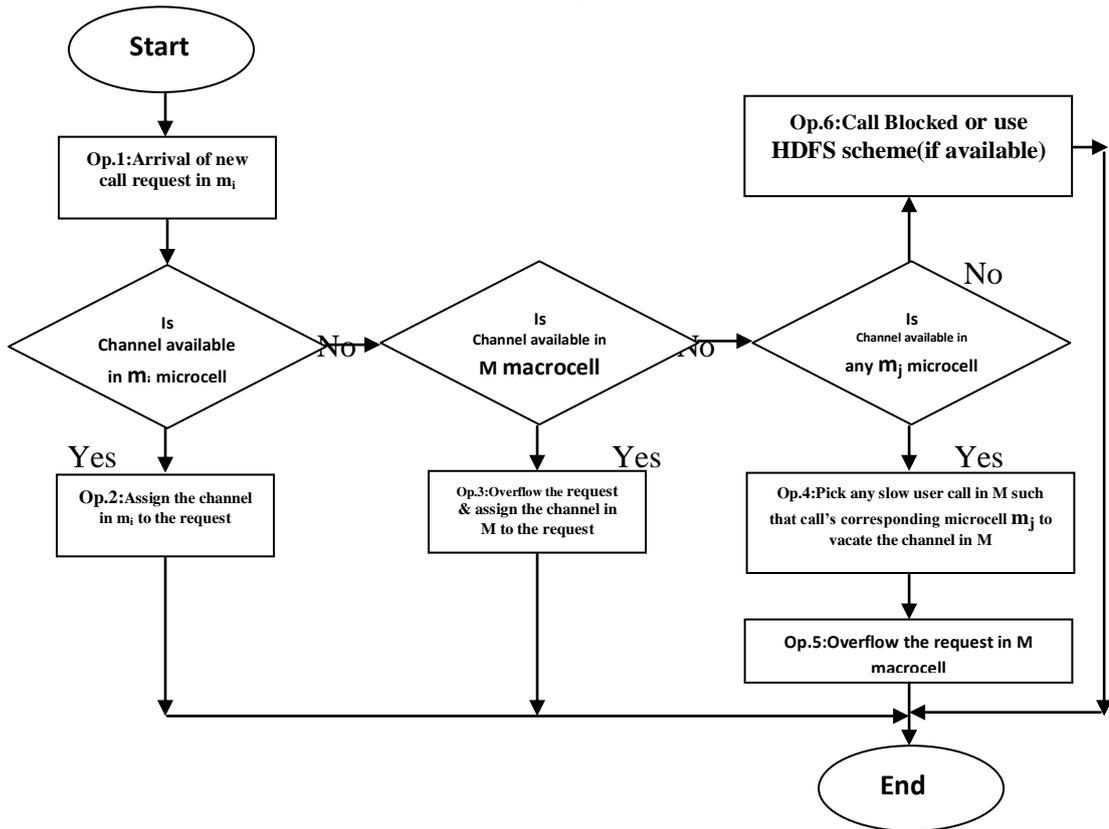
Figure 1: Flowchart 'A' showing Operations occurred on Call request arrived to microcell
