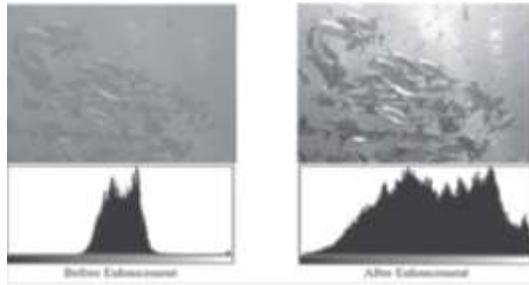
Figure 5: Comparison of results before and after enhancement (Kashif Iqbal et al., 2007)
