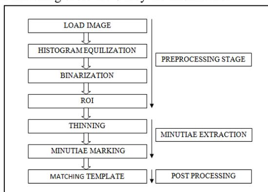
Fig. 2 Fingerprint Matching block diagram
