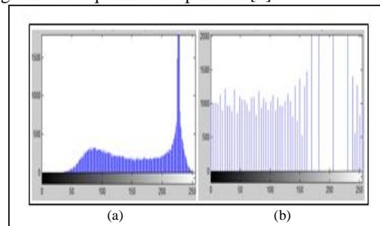
Fig. 3 (a) Original Histogram, (b) Histogram after Equalization
