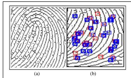
Fig. 7 (a) Thinned Image, (b) Extracted Minutiae in ROI
