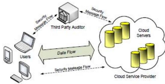
Fig. 1: The architecture of cloud data storage service
