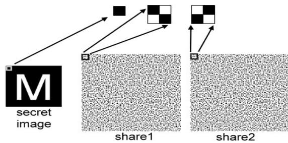
Fig. 1 An Ordinary (2, 2) Visual Cryptography scheme
