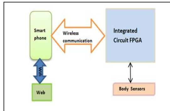
Fig.1 Block diagram of I-healthcare system
