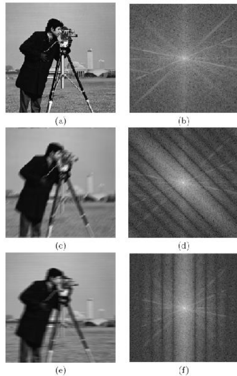
Fig 3: (a), (b) The original image and its Fourier spectrum. (c) The blurred image with motion orientation 45\pm and motion length 10 pixels. (d) Fourier spectrum of image (c). (e) Image blurred with motion length of 10\pm pixels and 0\pm orientation. (f) The Fourier spectrum of image (e).
