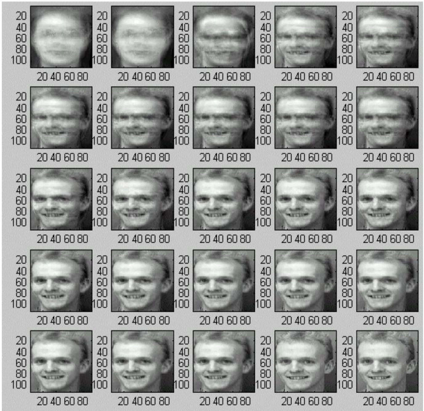
Fig 5 Reconstruction of first image with the number of Eigen Faces
