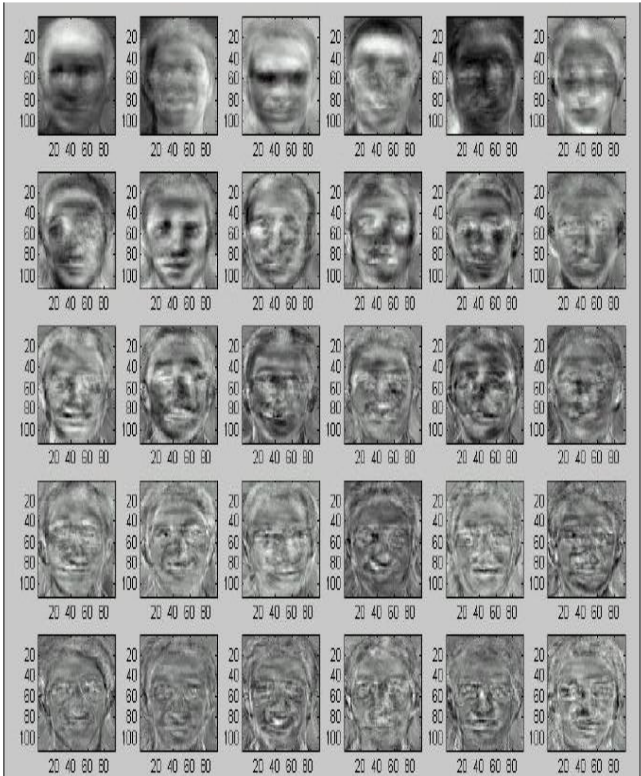
Figure 5.4 The top 30 eigen faces for the ORL Face Database
