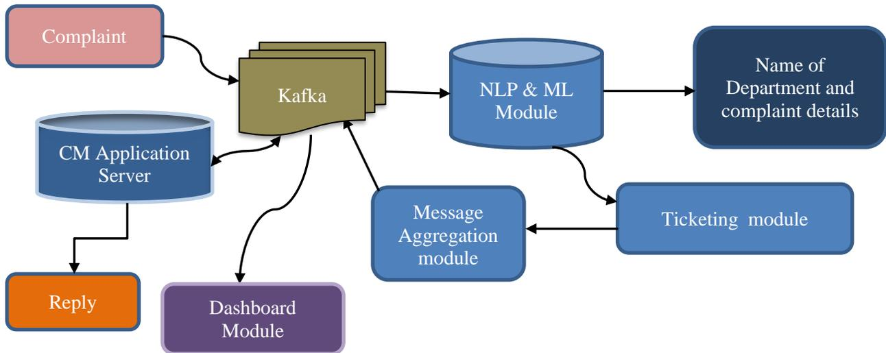
Fig. 1 System Architecture
