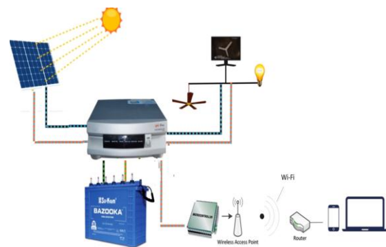
Fig 1: Functional Architecture of the Proposed IoT Based Smart Controlled Inverter
