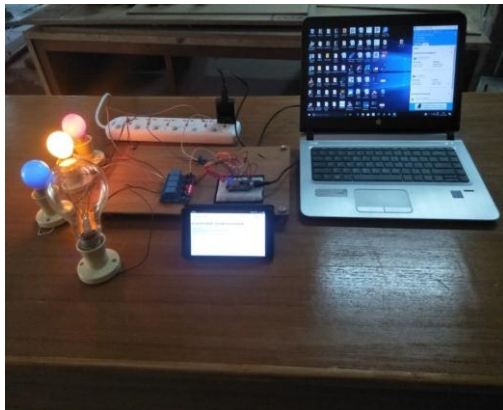
Fig 11: Web URL based remote control of equal three AC loads
