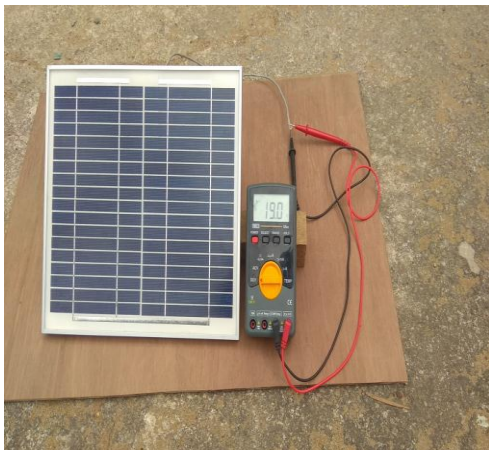
Fig 5: Acquisition of Green DC potential from 10w peak PV panel
