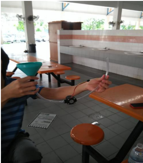
Figure 5.1 Location of the water flow sensor in piping system of the project (0°)
