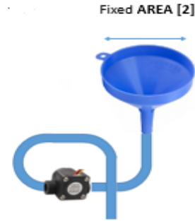
Figure 4.6 Rain Water Collection Dock
