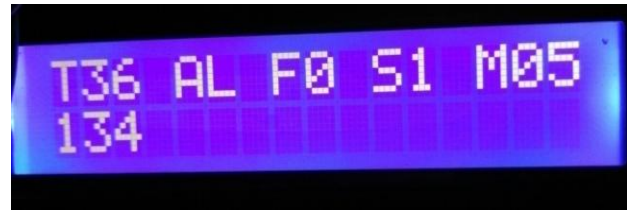
Figure 4: Temperature, Accelerometer, Frontobstacle, and Mistake indication
