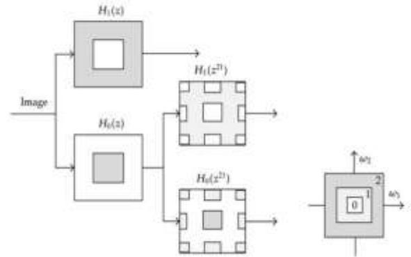
Figure 3 Nonsubsampled Pyramid (a) Three-stage pyramid decomposition. (b) Sub-band frequency plane.
