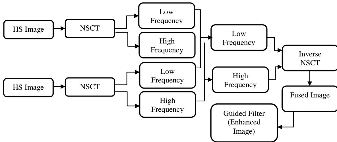
Figure 1 Block Diagram for fusing two images using NSCT and Guided Filter
