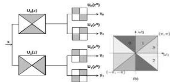
Figure 4 Nonsubsampled directional filter bank constructed with two-channel fan filter banks. (a) Filtering structure. (b) Corresponding frequency decomposition
