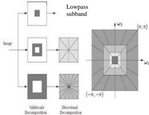
Figure 2 Non-sub-sampled Counterlet Transform. (a) NSF structure that implement NSCT.
