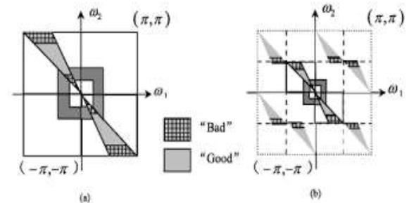
Figure 5 Sampling in the NSCT. (a) With no upsampling. (b) With upsampling.
