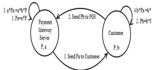
Fig. 8. Key exchange between PGS and Customer
