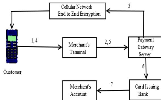
Fig. 3. Onsite Electronic Transaction
