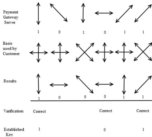
Fig. 9. Key distribution by PGS to customer by Quantum key distribution
