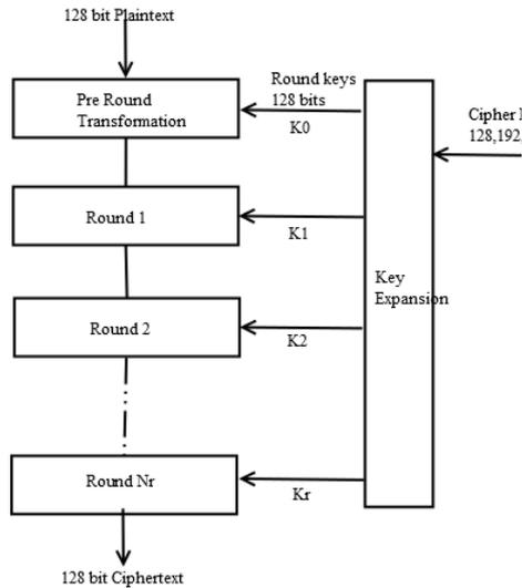
Fig. 2. AES Encryption Algorithm
