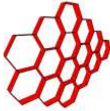
Fig. 8. Design 5, hexas without intersection simulating a honeycomb structure.
