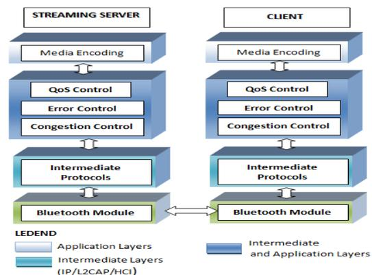
Fig. 8 Data Streaming Architecture
