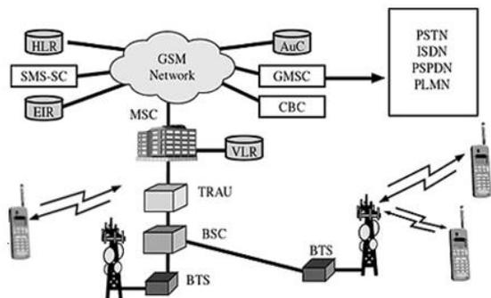
Fig. 5 GSM Architecture
