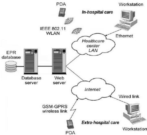
Fig. 4 System Overall Architecture
