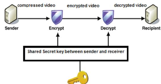
Fig. 10 Symmetric Key Encryption Technique
