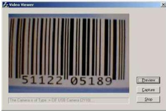
Fig. 5 Capturing barcode via USB webcam
