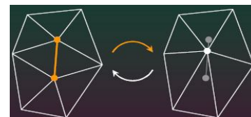
Figure 4. Separation of vertices (white arrow) and contraction of edges (red arrow)
