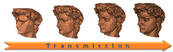
Figure 3. Progressive transmission of 3D object
