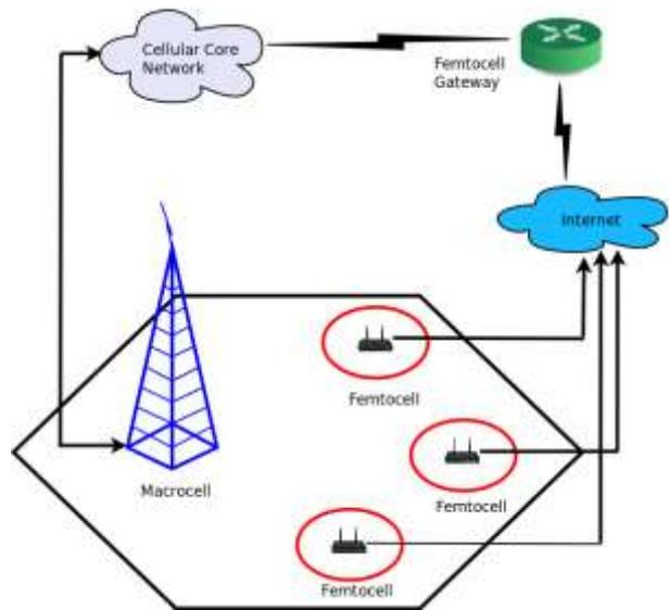
Fig. 1: Femtocell Architecture
