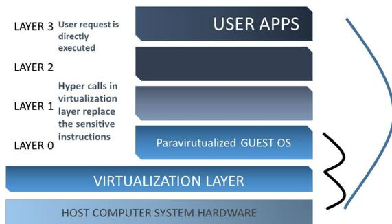
Fig-5 schematic of paravirtualization process
