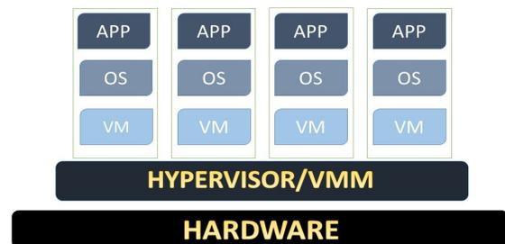
Fig 2- Virtualization process in cloud computing
