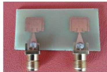
**Fig:3.2 Proto Type antenna (a) Front View**
