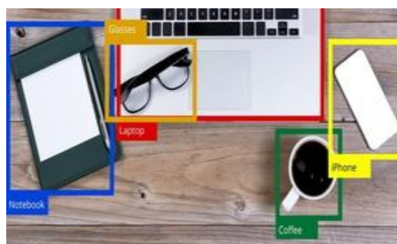
Fig 1: Object Detection Using Bounding Boxes
