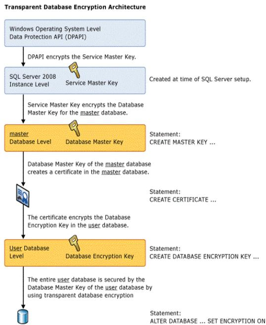
Fig 1: Transparent Data Encryption Process [2]
