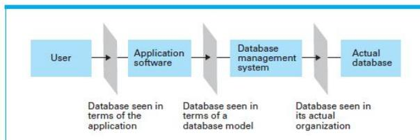
Fig. 2 The conceptual layers of a database management
