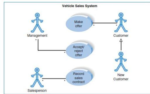
Fig. 8 Use Case Diagram With Specialized Actor
