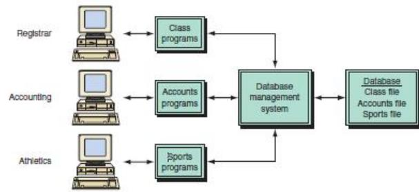
Fig. 3 The conceptual layers of a database management
