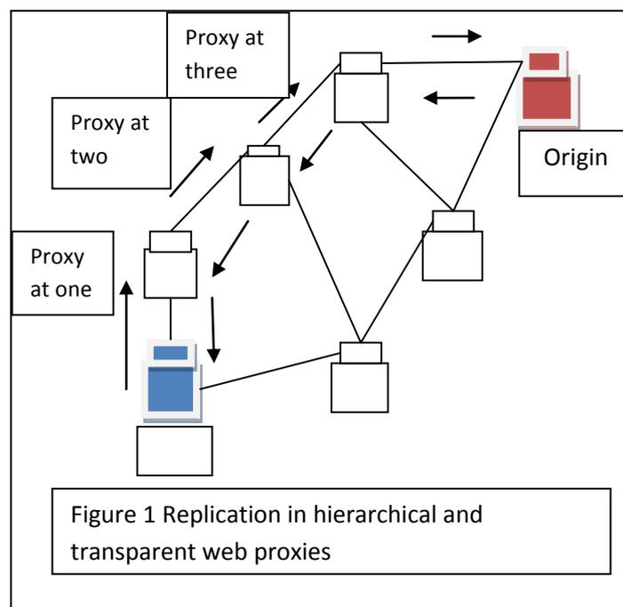
The server that contains the replicated data on behalf of an origin server is called as proxy server. It is selected based on various factors such as hop distance from client, reliability of the communication link and history of server crash or failure. The proxy server is selected for a client based on the above criteria. Replicating data object at different level of hierarchy increases availability and response time. At the other side more overhead
