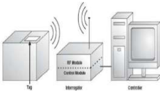
Fig. 1 Basic components of RFID
