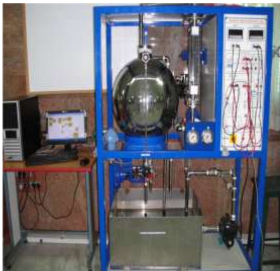
Fig.1 Real time experimental setup of a spherical tank
