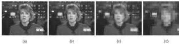
Fig 9 : (a) n = 1, original image. (b) n = 4. (c) n = 8. (d) n = 16. Original and corresponding low resolution images. Each square cell consists of n x n pixels in which the intensity of each pixel is replaced by the average intensity of the pixels in that cell.
