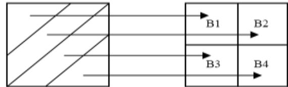
Fig. 2 Mapping of DCT coefficients into 4 blocks
