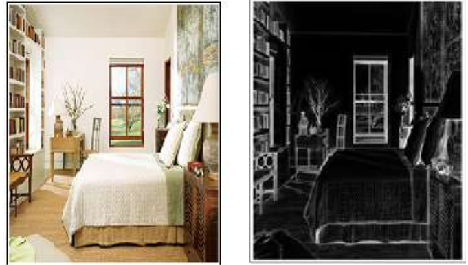
Fig. 2: An example of bedroom image taken from MIT-indoor dataset and its corresponding morphological gradient.
